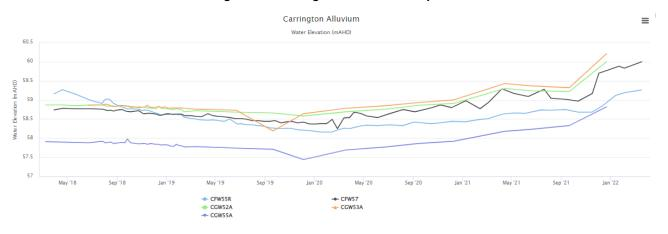
Figure 29 - Carrington Alluvium Water Elevation Trend - Q1 2022
