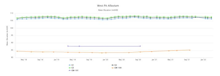
Figure 62 - West Pit Alluvium Water Elevation Trend - Q1 2022
