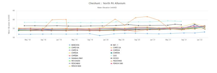
Figure 41 - Cheshunt North Pit Alluvium Water Elevation Trend – Q1 2022
